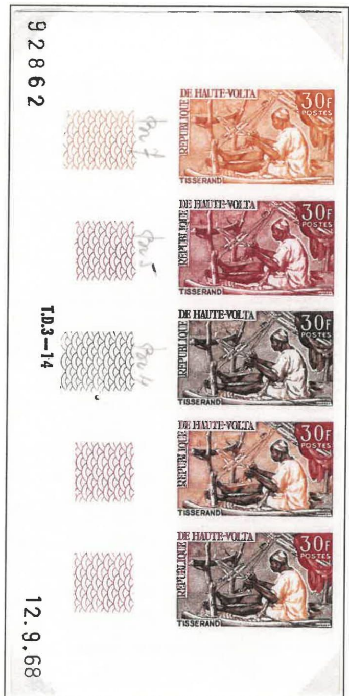
A colour sample of the Upper Volta stamp of 1968. The edges of the sheet are marked with the code of the respective colour (handwritten annotations), the sheet number, the number of the printing press and the date of printing.
